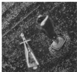
Fig. 9. Silicon p-n-p pellets with \sim 0.003 in. bases. Emitter and collector etched.
