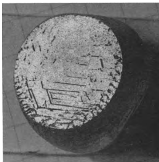
Fig. 4. Surface cut perpendicular to the growth axis from a heavily doped vertical crystal similar to that shown in Fig. 3. The surface was cut just above the region where randomly oriented polycrystal development starts. Note how the excess Bi was deposited along (1,1,1) planes in this region during growth and has been removed in the subsequent etching of this surface.
