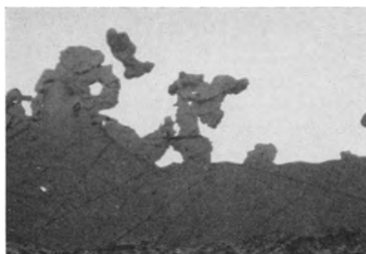
Fig. 8. Metallographic cross section of magnesium anode: polarization current = 100 \mu\text{a cm}^{-2} ; temperature = 75^\circ\text{C} ; time = 7 days; solution = 110 ppm NaCl. Magnification 150X before reduction for publication.
