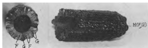
Fig. 3. Lead dioxide of the mixed texture of fiber and granule; F, fiber; G, granule.
