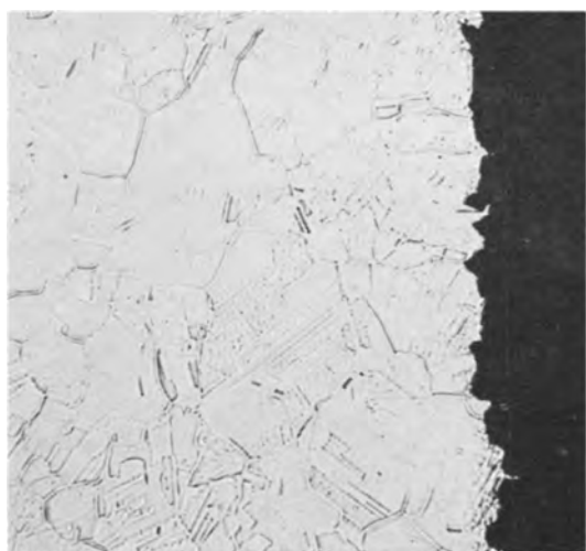
Fig. 2. Section perpendicular to the surface of a silver electrode from which silver was dissolved anodically. Magnification 500X.
