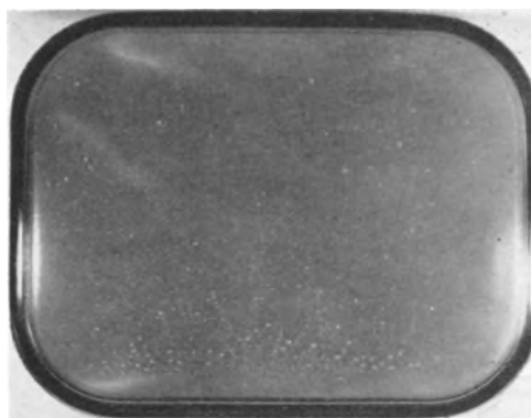
Fig. 5. Effect of the addition of surface active agents to lacquer showing the nonwetting of the moistened screen by the lacquer.
