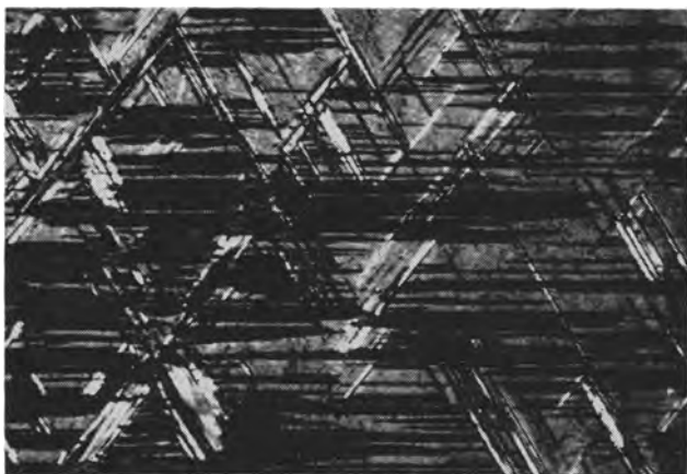
Fig. 6. Nitride platelets on a polished surface viewed under polarized light. Specimen treated as in Fig. 5. Magnification 500X before reduction for publication.
