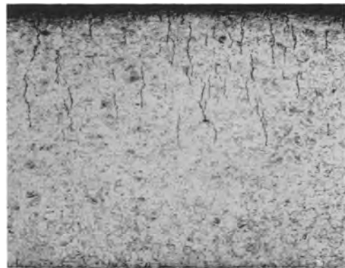
Fig. 7. Sheared edge of bent, stress-relieved specimen after 8-min exposure to 42% MgCl 2 . Electrolytic etch, 50X.
