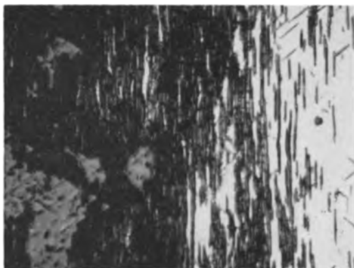
Fig. 4. Taper section of oxidized single crystal surface. 500X before reduction for publication.
