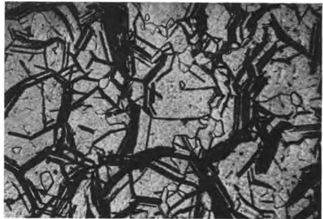
Fig. 4. \beta -TaH precipitate in fine-grained Ta sheet. Treatment, 24 hr, 700°C in H 2 . Magnification 500X before reduction for publication.
