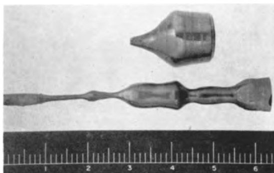
Fig. 6. Crystals of AlSb grown from the melt
