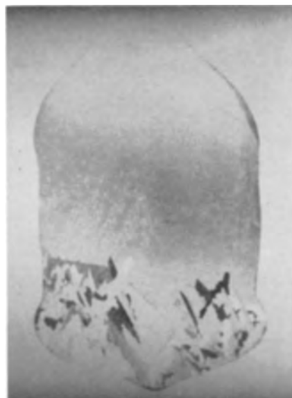
Fig. 3. Cross section from top to bottom of a vertically pulled ingot of Ge. The quantity of doping impurity added to the initial melt was so chosen that it would increase sufficiently in concentration to affect noticeably the perfection when approximately half the crystal was pulled. The gross imperfections in the center region and the polycrystal bottom were brought out by etching in silver etch.
