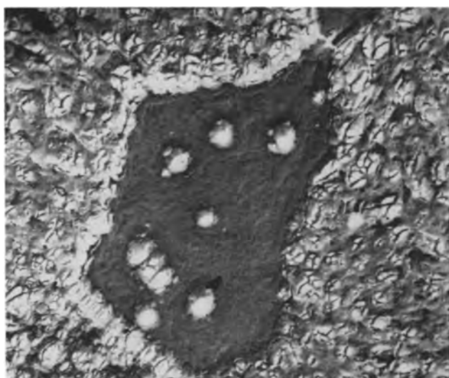
Fig. 2c. Formvar replica, shadowed with gold-Manganin, of Nb specimen oxidized for 210 min at 400°C. Magnification 5,000X before reduction for publication.
