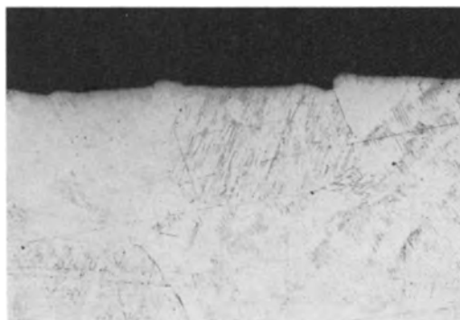
Fig. 9. Metallographic cross section of magnesium electrode demonstrating acid attack, etched. Magnification 150X before reduction for publication.
