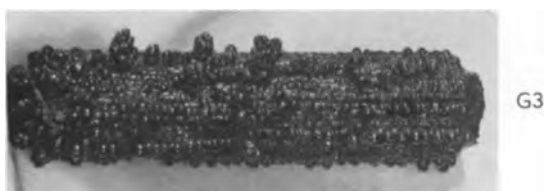
Fig. 7. Electrodeposited lead dioxide whose granules were formed on projected points of the substrate. The substrate was shaped by hand with a knife to a cylindrical rod. There was many stripes parallel to the axis on the surface of the substrate.
