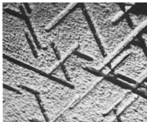
Fig. 3. Traces of the \{100\} planes. 2000X before reduction for publication.
