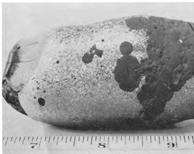
Fig. 6. Typical boron deposit (Scale in inches)
