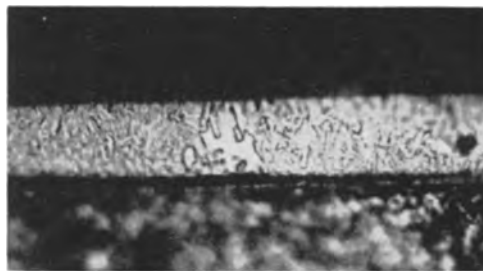
Fig. 6. Initial status of grain growth, after direct stress of \pm 18 kg/mm 2 for 9 \times 10^5 cycles (1000X).
