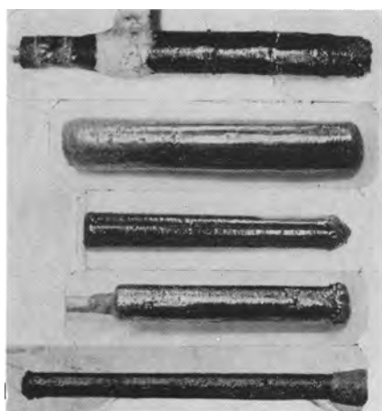
Fig. 2. Hollow cylinders of bright, smooth lead dioxide, from top to bottom: BS1, BS4, BS5, BS6, and BS7.
