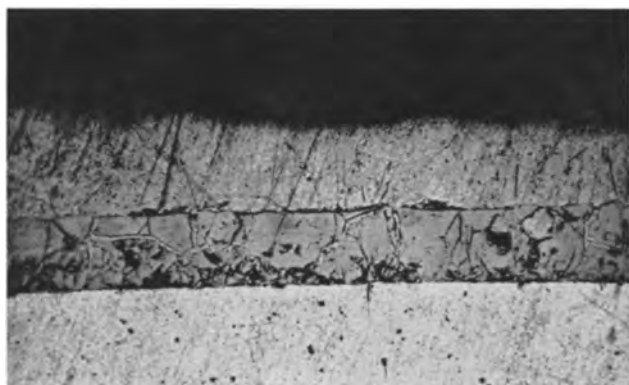
Fig. 13. Photomicrograph of a typical iron-molybdenum deposit. Magnification 500X before reduction for publication.
