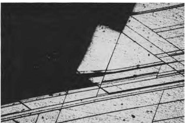
Fig. 7. Fracture associated with the nitride-metal interface
