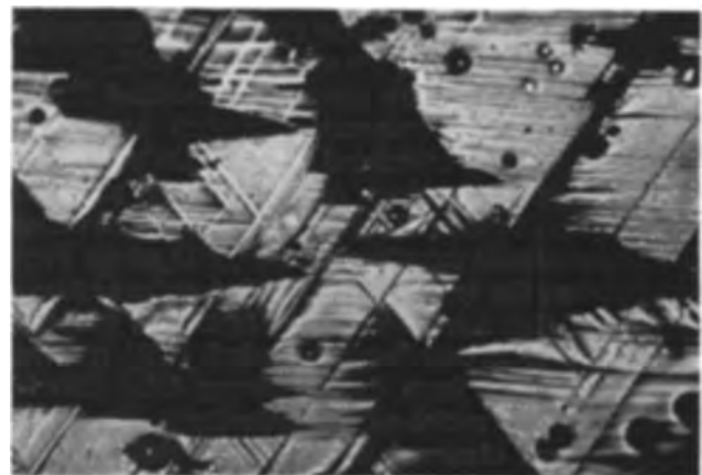
Fig. 5. Surface nitride (dark material) and distortion resulting from nitride precipitation on the {100} planes on a single crystal of Ta after 24 hr at 750°C in N 2 atmosphere. Magnification 500X before reduction for publication.
