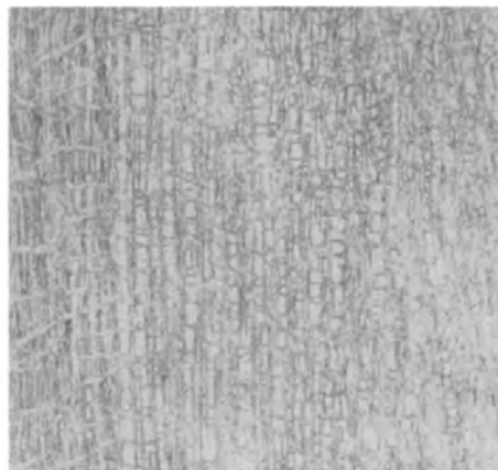
Fig. 6. Niobium containing 0.20 H/Nb quenched from equilibrium at 500°C. Magnification, 250X before reduction for publication.
