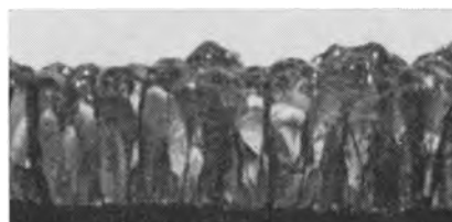
Fig. 4. Broken surface of columnar lead dioxide: C
