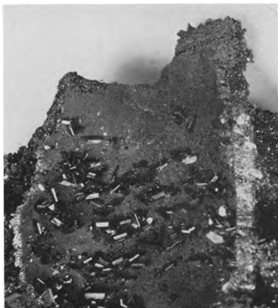
Fig. 2. SiC crystals on a graphite substrate. Magnification 2X.
