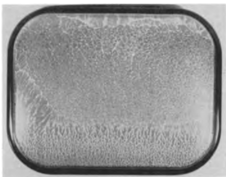
Fig. 1. General appearance of lace pattern in the lacquer film on a 14-in. screen.
