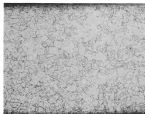
Fig. 13. Sheared edge of unbent specimen, annealed 1050°C, W.Q., exposed to 42% MgCl_2 for 2 hr. Electrolytic etch, 50X.
