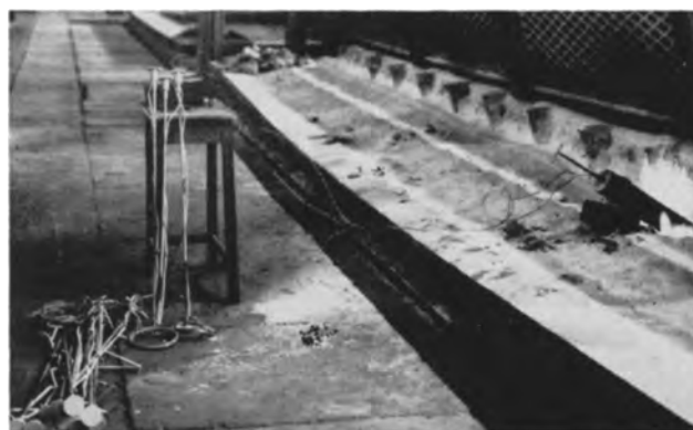
Fig. 2. Apparatus for measuring magnetic field directions in furnace baths set up beside a 100 KA furnace. To the base of the aluminum cylinders are attached asbestos disks to keep the cylinders central in the graphite tube which is shown inserted under the anode. A protected search coil is inserted into the tube to measure field strength.
