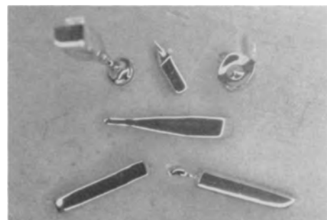
Fig. 7. Germanium p-n-p pellets. Top left, emitter etched; top right, emitter etched off; center, nonselective attack at higher voltages; bottom right, collector etched; bottom left, collector etched off.
