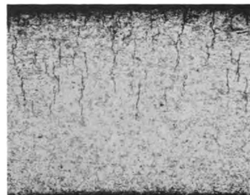
Fig. 8. Sheared edge of bent, stress-relieved specimen after 10-min exposure to 42% MgCl 2 . Electrolytic etch, 50X.
