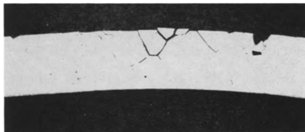
Fig. 13. Stressed Al-4% Cu binary alloy after exposure to 53 g/l NaCl with 12 ma anodic current for 4½ min.
