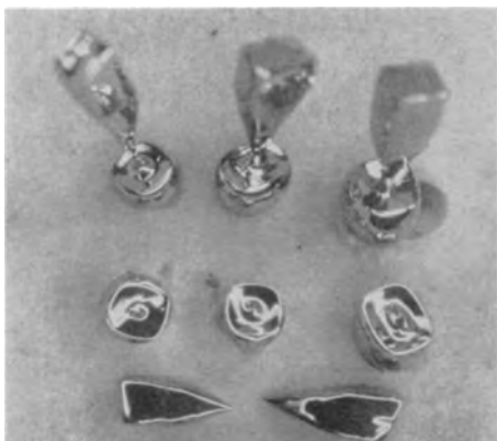
Fig. 8. Silicon p-n-p pellets. Top, emitter etched; center and bottom, emitter etched off.
