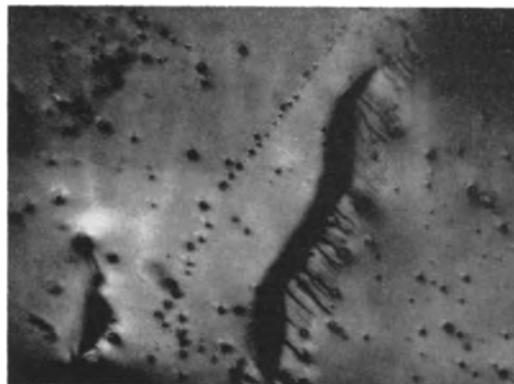
Fig. 7. Fractograph showing sites of nucleation of oxygen metal reaction on a grain surface. 500X before reduction for publication.
